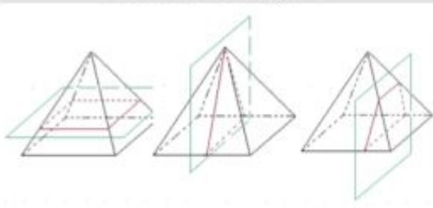
Cross-section is another name for a plane section, but often that name is reserved for a section of a three-dimensional object that is parallel to one of its planes of symmetry or perpendicular to one of its lines of symmetry. So, for example, for a cube, one line of symmetry joins the centers of opposite faces. A cross-section perpendicular to that line is a square, as is the cross-section of the right rectangular pyramid shown above left.
